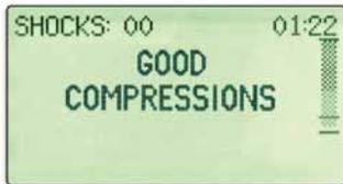
during cardiopulmonary resuscitation (CPR). In addition to audio prompts, both the AED Plus and AED Pro feature on-screen instructions, and a bar gauge that shows how deep to push in order to optimize compression depth. This is an important advance, given the American Heart Association’s 2010 Guidelines and their recommendation for chest compressions at least two inches deep.
